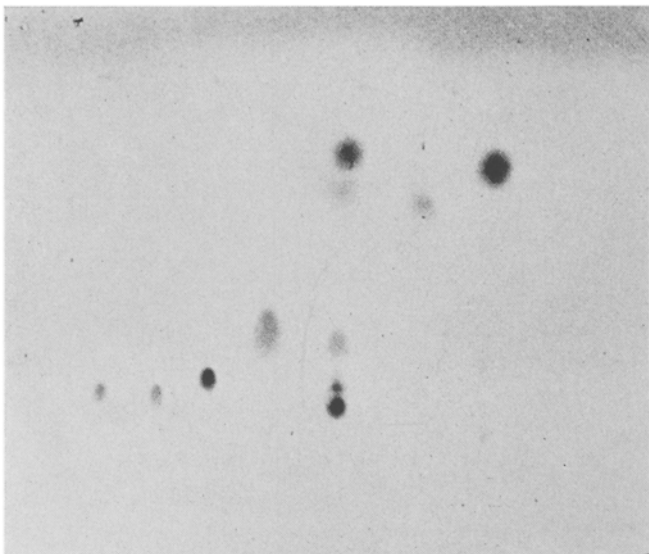
FIG. 2. Chromatogram showing the position of six divinyl monomers and a synthetic mixture of these on direct plate, the solvent system being n -hexane-ether (100:5 v/v); from left to right: diallyl sebacate, 1,10-diacryloxydecane, 1,10-dimethacryloxydecane, divinylsebacate, synthetic mixture, 1,10-diallyloxydecane and 1,10-divinyloxydecane.
